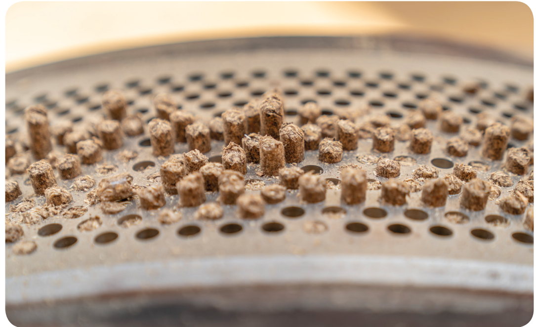
Figure 5: Fiber being pushed through a die to form a wood pellet.
