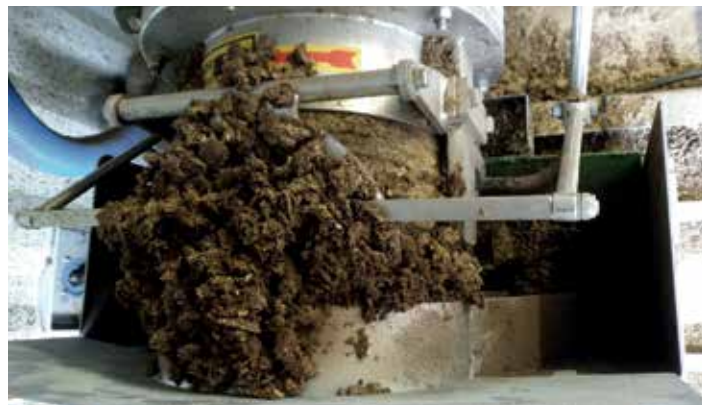
Figure 3. Solid digestate from behind the dewatering with a screw press separator. This falls onto the conveyor belt of the disputable dryer
